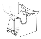
If leak occurs, check to make sure all connections are properly sealed. Contact Bemis support for assistance.
