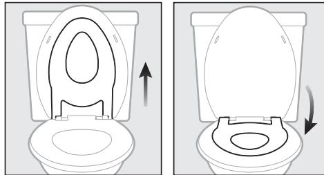
**To position the child seat for use, lift child seat straight up and lower.**
