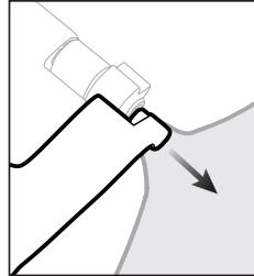
**To disengage child seat, pull one side away from the hinge.**
