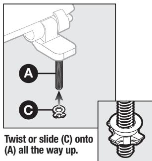
**Twist or slide (C) onto (A) all the way up.**
