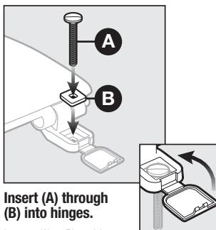
**Insert (A) through (B) into hinges.**
