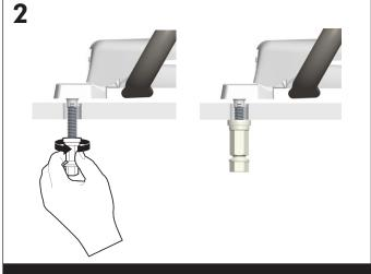
Lightly finger tighten both Snap 2 Secure nuts
