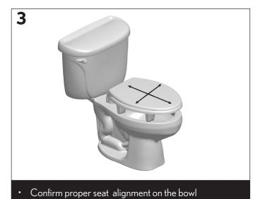
If not properly aligned, adjust seat and hold in place
